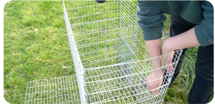
2) Fold down the inside fence to 90 degrees and secure with zip ties.
